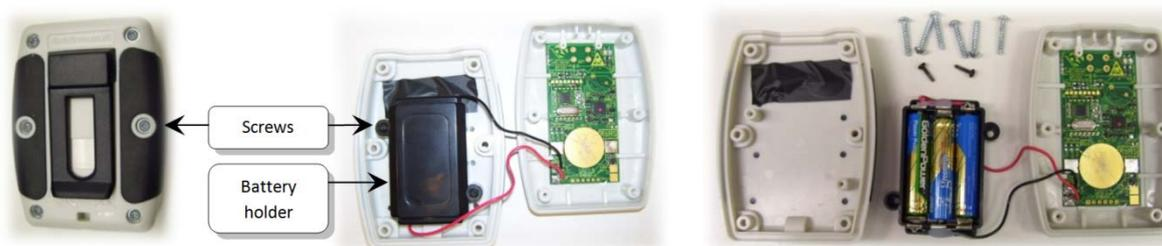
**Figure 2: Battery replacement**
