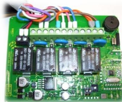
Figure 7: Receiver PCB
